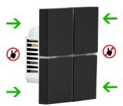
For installing or removing the faceplate, please are care that only pushes corners. Do not push the side middle, it may damage this product. Look at the picture, green arrow shows that where must be pushed out for removal or push in for install.
